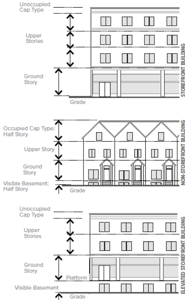
Figure 27-15.20.10 A. Measuring Building Height
